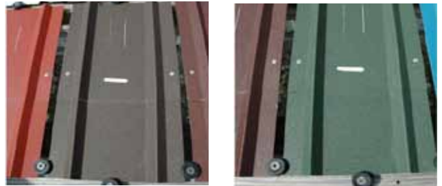
Figure 2: ArcelorMittal Dofasco exterior exposure (weathering) testing program
